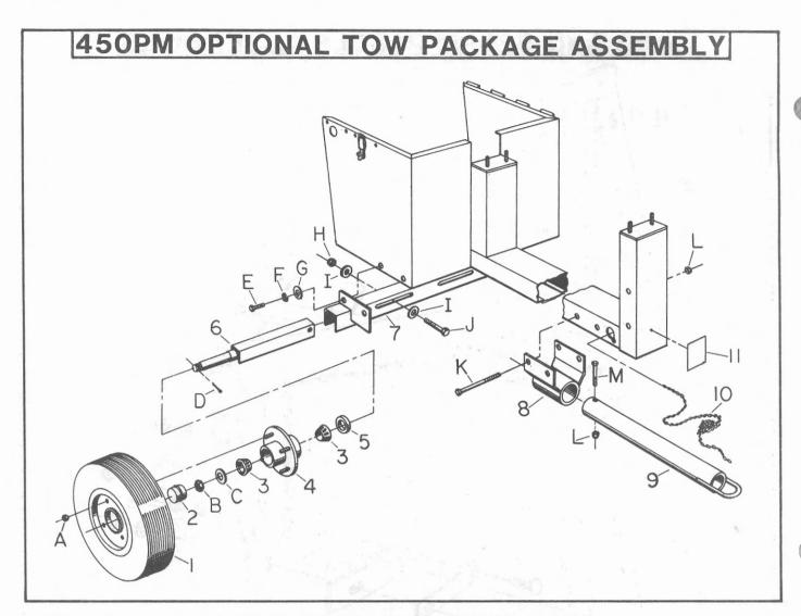
WARNING - DO NOT ATTEMPT TO TOW ANY 450PM MIXER NOT EQUIPPED WITH THE OPTIONAL TOWING PACKAGE ILLUSTRATED HERE. CONSULT THE TOWING SECTION IN THE FRONT OF THIS MANUAL FOR ADDITIONAL SAFETY PRECAUTIONS.
